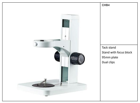
CHB4 Track Stand Vertical Height: 300mm Mounting Size: Φ76mm Focusing Distance: 106mm With φ95mm B/W Plastic Plate and Paired Clips Base Size: 200x255x22mm
